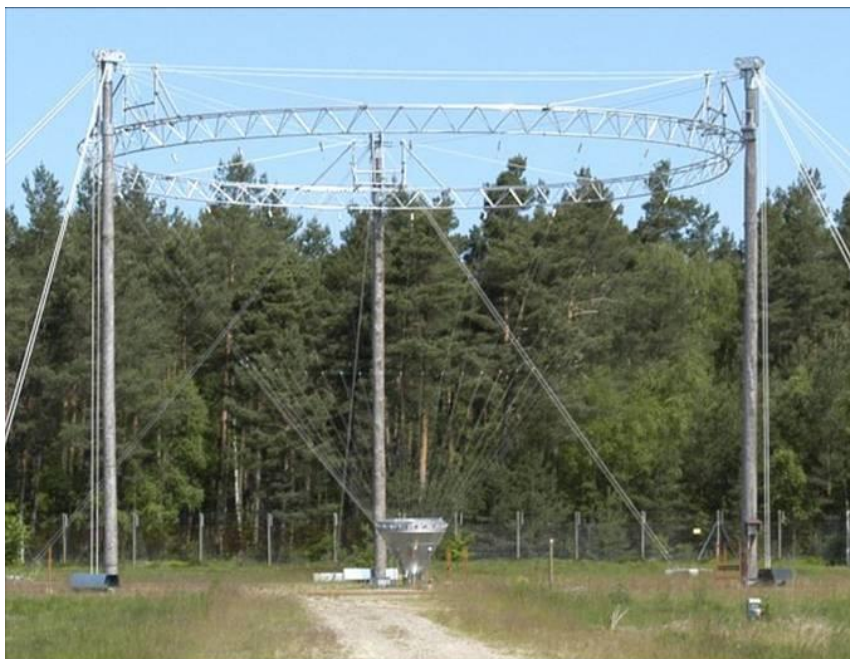
Figure 505-10: Illustration of a Vertically Polarised NEMP Simulator
